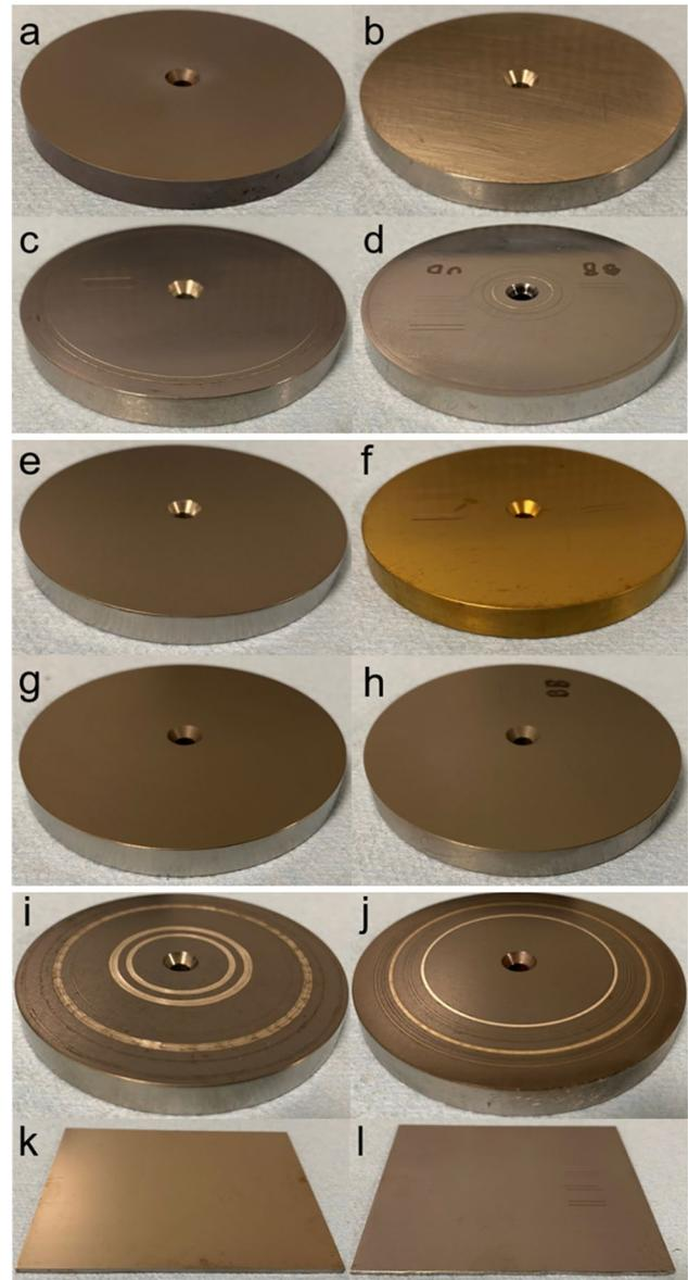
**Fig. 2** Photos of the samples tested in this study: **a** 440C with MS 200-1, **b** Nitronic 60, **c** Nitronic 60 with MS 200-1, **d** EDM Ti6Al4V with MoS<sub>2</sub>, **e** Anodized Ti6Al4V (Danco Type 2), **f** Nitrided Ti6Al4V, **g** Anodized Ti6Al4V (Tiodize Type II), **h** Anodized Ti6Al4V (Tiodize Type IV), **i** Ti6Al4V with i-Kote, **j** 440C with i-Kote, **k** Ti6Al4V, and **l** Ti6Al4V with MS 200-1
