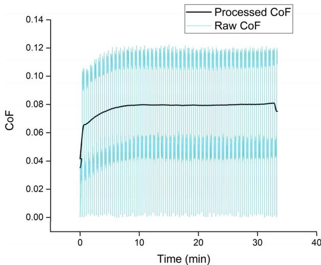
**Fig. 3** CoF plot from a linear reciprocating test showing raw and processed data
